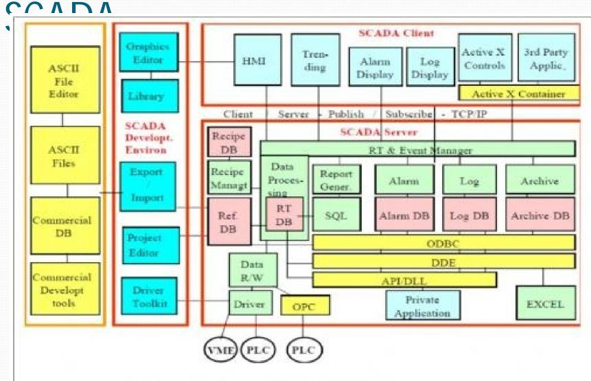
Typical generic software architecture of SCADA systems
